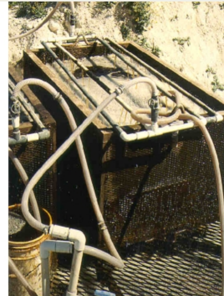
Compost tea brewing: pumping, trickling, aeration, California
