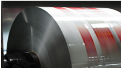
Giant roll of flexible laminate shipped to filling plant, pouches made and filled in one operation
